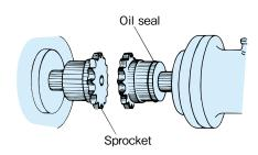
Bring the sprocket faces close together and correct the angular and parallel misalignment.
