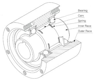
The figure shows a representative model from the MZ Series for explaining construction.
