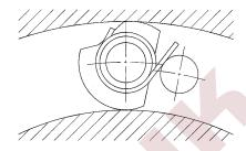
Figure 1: Entire Cam Clutch is stationary
