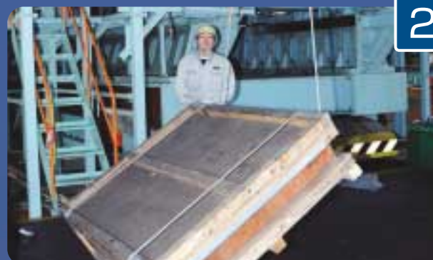
Stand wooden box upright when removing chain. (Be careful when standing wooden box.)
