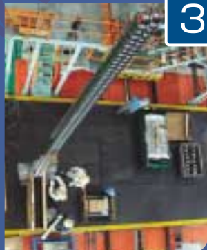
Chain is packaged folded on top of itself. Attach one end to a crane and lift out for easy removal.
